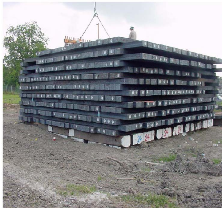
Photograph 2. Cell A fully loaded with 1 million kilograms of steel (177 kN/m 2 ).
